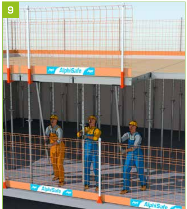
- While holding the panels in place, prop up the panels as per the MaxiDalle user guide.
