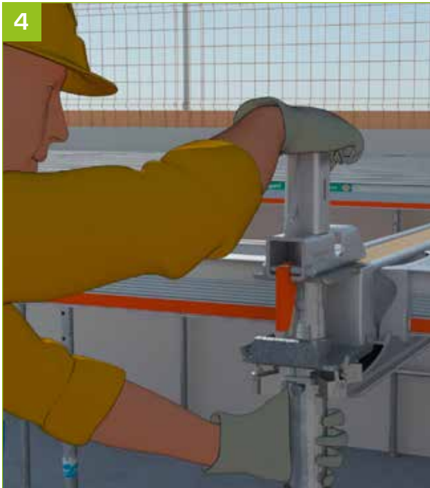
- The adapter anti-dropout system locks automatically onto the prop.
