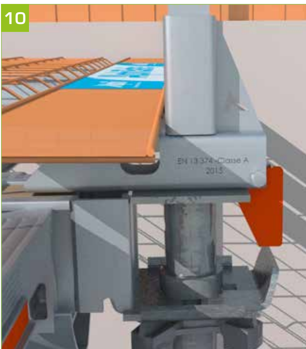
- Move the AlphaSafe mesh so that the baseboard is in contact with the AlphaSafe adapter.
