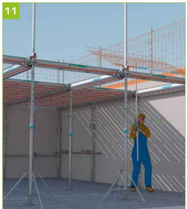
- From the work surface, simply lift the AlphaSafe mesh using the AlphaSafe pole.
