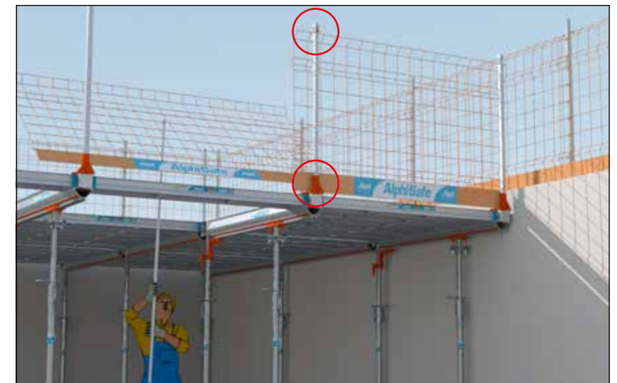
- The grid is locked at the top by the anti-lifting pin and is locked at the base.
