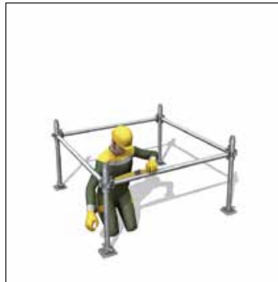
- Location and levelling.
