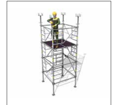
- Set up and adjust the head jacks.
